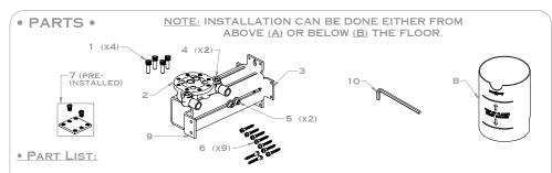
1. MANIFOLD BOLTS (X4) 2. MANIFOLD ASSEMBLY (1/2 "NPT) 3. MANIFOLD MOUNTING BRACKETS 4. MANIFOLD STOPS (X2) 5. EXTENSION ARM BOLTS (X2) 6. MOUNTING BRACKET SCREWS (X9) 7. MANIFOLD MOUNTING PLATE & SCREWS (X2) 8. ROUGH COVER 9. EXTENSION ARMS 10. 1/4" ALLEN KEY
