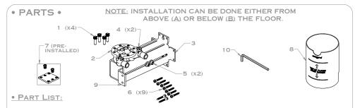
1. MANIFOLD BOLTS (X4)2. MANIFOLD ASSEMBLY (1/2 "NPT)3. MANIFOLD MOUNTINGBRACKETS4. MANIFOLD STOPS (X2)5. EXTENSION ARM BOLTS (X2)6. MOUNTINGBRACKET SCREWS (X9)7. MANIFOLD MOUNTING PLATE & SCREWS (X2)8. ROUGH COVER9. EXTENSION ARMS10. 1/4" ALLEN KEY
