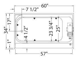
(  $\blacktriangle$  ): Indicates Whirlpool jets positioning (  $\triangle$  ): Indicates suction positioning
