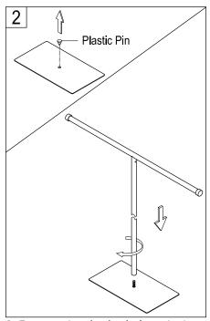
2. Remove the plastic pin from the base. Place the base assembly on a level spot on the ground. Thread the free end onto the base assembly tightly in a clockwise direction and use the provided gaskets to cover the exposed corners of the bottom of the base. Check that all bolts are tight and secure on your completed towel holder.
