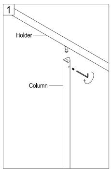
1. Install the holder into the column, attach it securely by tightening the set screw with an Allen wrench.
