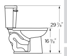
THIS FIXTURE QUALIFIES ACCORDING TO ASME TEST PROCEDURES AS A HIGH EFFICIENCY WATER CLOSET WITH AN AVERAGE CONSUMPTION OF 1.28 gpf (4.8 Lpf) OR LESS.
